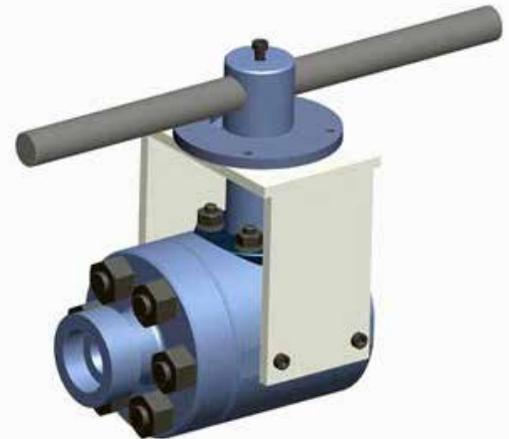
*The solution included: three 2-inch EVS 1500 pound, 1.5-inch bore F22 body socket-welded, metal-seated ball valves; attached to Field Q QD600 actuators (not shown in drawing above); fitted with Asco solenoids; and Topworx limit switches for each unit.*
