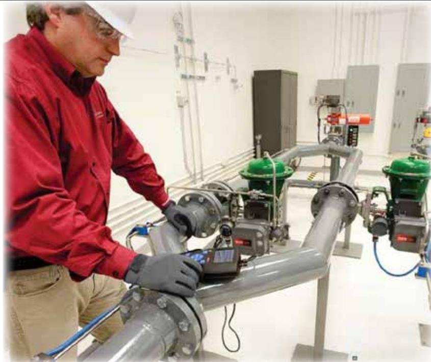
At the Fisher testing facility, a technician uses advanced diagnostic equipment to certify the condition of Vee-Ball control valves fitted with FIELDVUE digital valve controllers.
