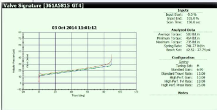
Sample test result screens from the Advanced Diagnostics scans on the Fisher Vee-Ball control valves.
