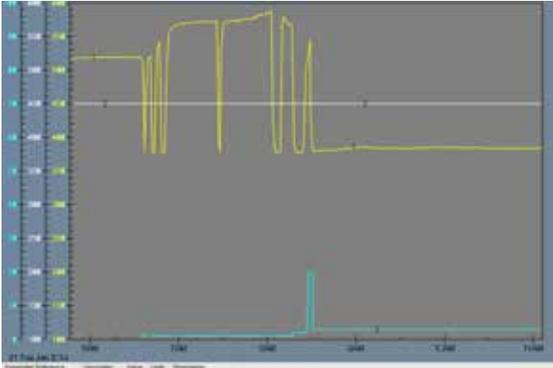
Above: spray water valve Cv performance before changes and, below, after replacement with the recommended 2-inch EZ with Microform Trim. Note the DeltaV screen shot above shows wide temperature swings between 380 and 490 F, versus the narrow range below after replacement, holding steadily around around the 425 F setpoint.
