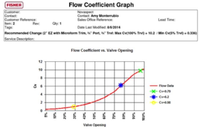
Above: performance chart of flow coefficient versus valve opening: existing spray water valve (2-inch EZ full port); below, improved performance of the same valve with the recommended trim change (2-inch EZ with Microform Trim, 3/4-inch port, 3/4-inch travel, maximum Cv (100% travel) equals 10.2 / minimum Cv (5% travel) equals 0.336).
