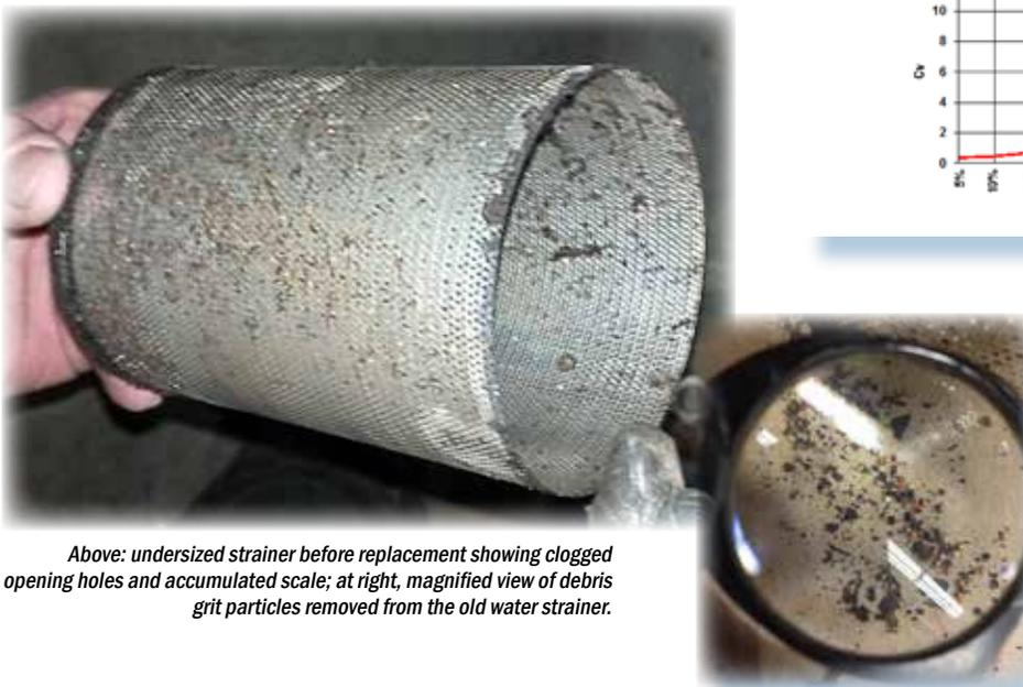
Above: undersized strainer before replacement showing clogged opening holes and accumulated scale; at right, magnified view of debris grit particles removed from the old water strainer.
