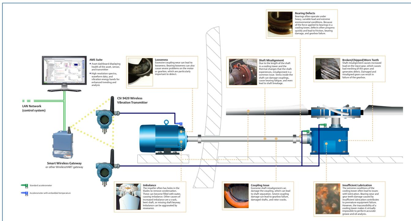
*A propeller fan, with its associated motor and gearbox, can be monitored remotely using wireless vibration transmitters and a gateway.*
