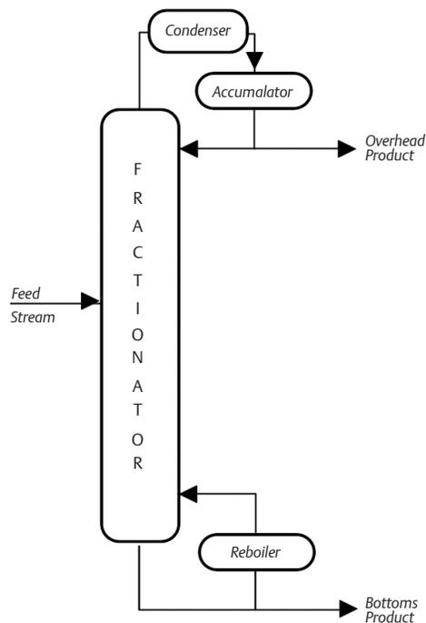
As the gases leave the top of the tower, they are cooled in a condenser, collected in an accumulator and then exit as the overhead product. To further increase the purity of the overhead stream, some of it is recycled (called reflux) for additional processing. The higher the reflux ratio, the purer the overhead product becomes.
