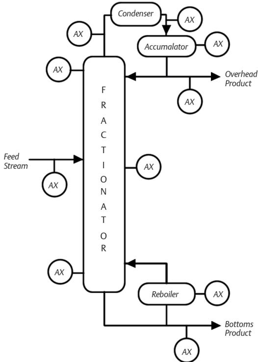
This is due to the fact that the tower separates by boiling point so if the concentration of one compound remains low, all the compounds that boil higher (or lower for the bottoms stream) will also be kept low. This compound is often referred to as the "key" compound – the light key and heavy key. If these are minimized, all the other impurities are also minimized.
