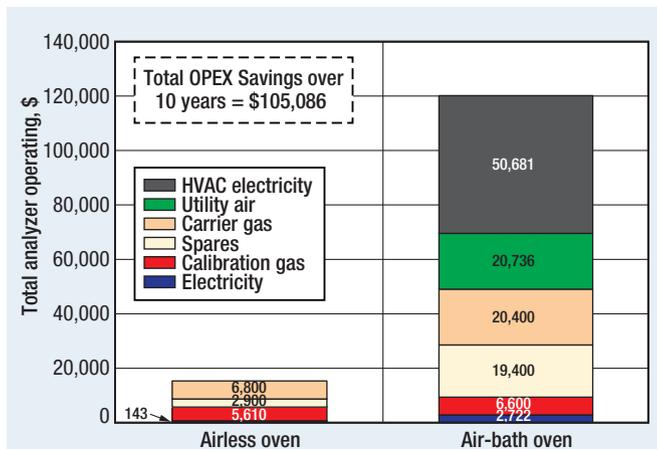
FIG. 4 Ten-year cost comparison of field-mountable and conventional process GC (1 GC).
