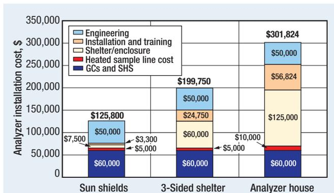
FIG. 3 Installation cost comparison of field-mountable and conventional process GC (1 GC).
