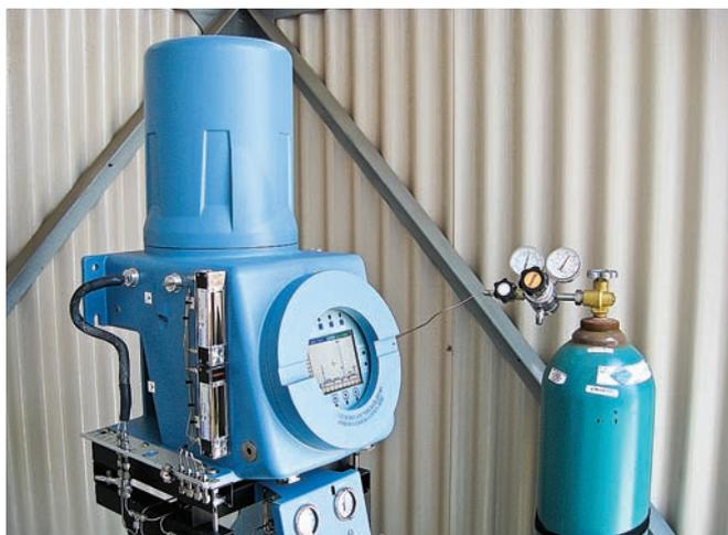
FIG. 2 Field-mountable process GC.
