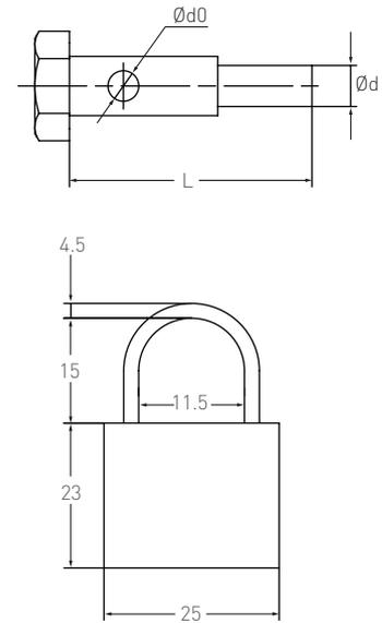
FIGURE 6 - LOCK PIN AND PAD LOCK (mm)
