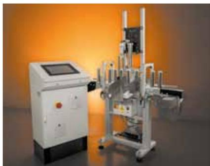
Emerson's Cascade CT2211 aerosol microleak detection system uses Quantum Cascade Laser (QCL) technology to instantaneously detect and reject leaking cans moving down the production line at a rate of up to 220 cans per minute.
