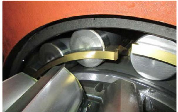
*Emerson’s Online Machinery Health Monitoring solution monitored the condition of a fracture in the gearbox’s bearings’ cage allowing safe production for 17 days.*
