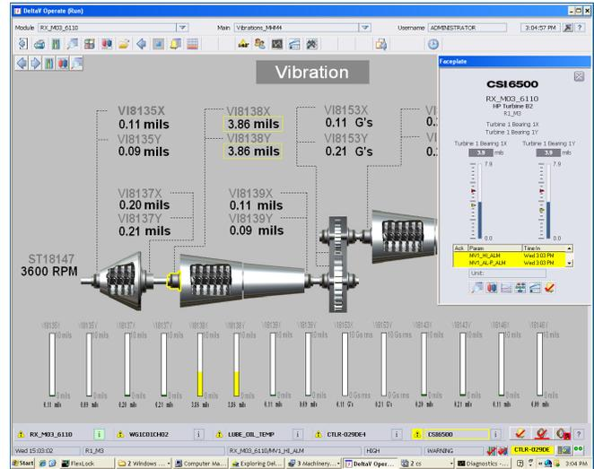
AMS 6500 faceplate and dynamos are included in DeltaV software. Dynamos allow users to drag and drop bargraphs and number elements on the screen to create graphics in no time — attach dynamo to the data point and you're done.
