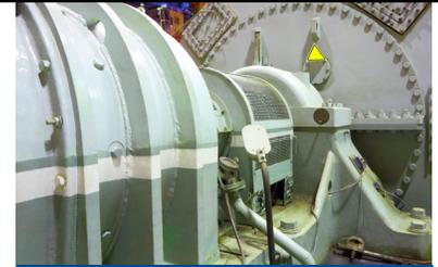
***Wireless temperature, pressure, and DP have been employed to check for hot air leaks, forced draft fan leaks and filter plugging. Online monitoring has enabled engineers to improve turbine efficiency and reduced megawatt use as well as extend the life of turbine fans.***
